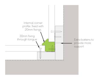
Fig. 7 - Internal corner detail
