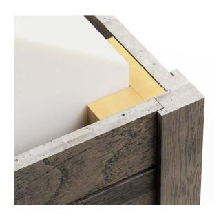
Alternatively, the boards can be butted together on an internal corner as shown in fig. 9. The boards can also be mitred to create the external corner, this would also be applicable if the corner is anything other than 90 degrees.
