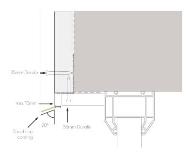
Fig. 15 - Window/door head with angled cut
