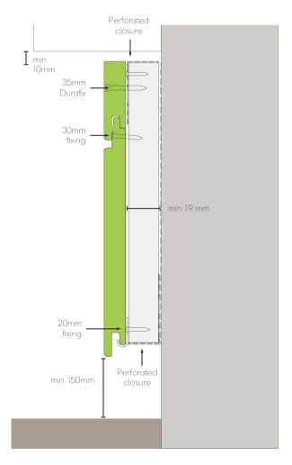
Fig.1 - Top & bottom cladding detail
