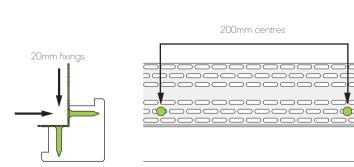
Fig. 6 - Use of perforated closure on corner profiles
