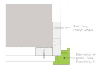
Fig. 8 - External corner detail
