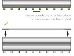
Lift boards on the edges using 2 people to lift at a time
