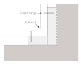
Fig. 9 - Internal butt jointed detail
