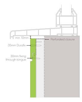
Fig. 3 - Window/door sill detail
