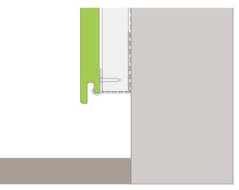
Fig. 17 - First board install
