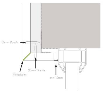
Fig. 14 - Window/door head with mitred joint
