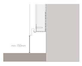
Fig. 4 - Install detail above ground level
