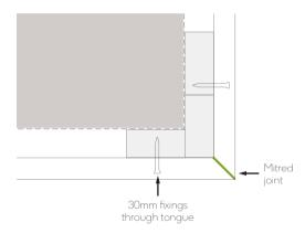
Fig. 10 - External mitred corner detail
