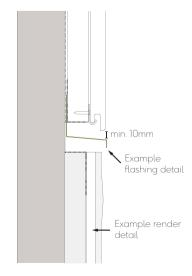
Fig. 21 - Installing cladding above render
