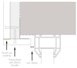
Fig. 12 - Window/door head with fascia
