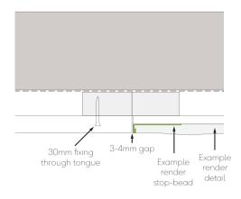
Fig. 19 - Corner profile butting upto render
