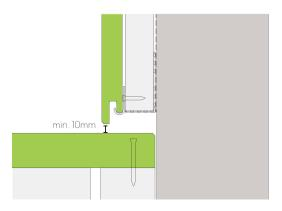
Fig. 5 - Install detail above deck
