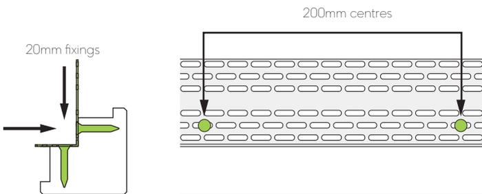
Fig. 6 - Use of perforated closure on corner profiles
