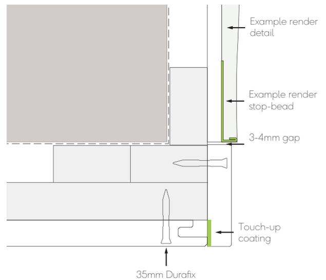
Fig. 20 - Corner profile butting up to render on external corner
