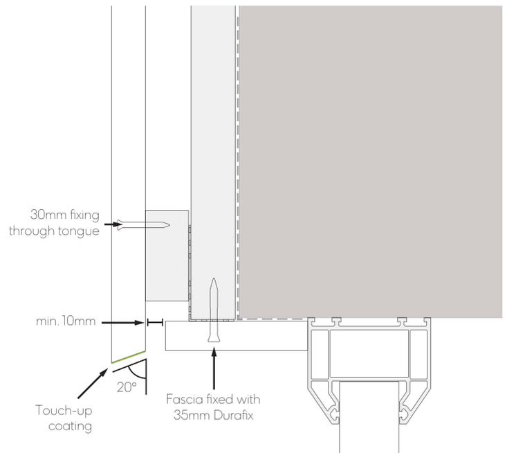
Fig. 15 - Window/door head with angled cut
