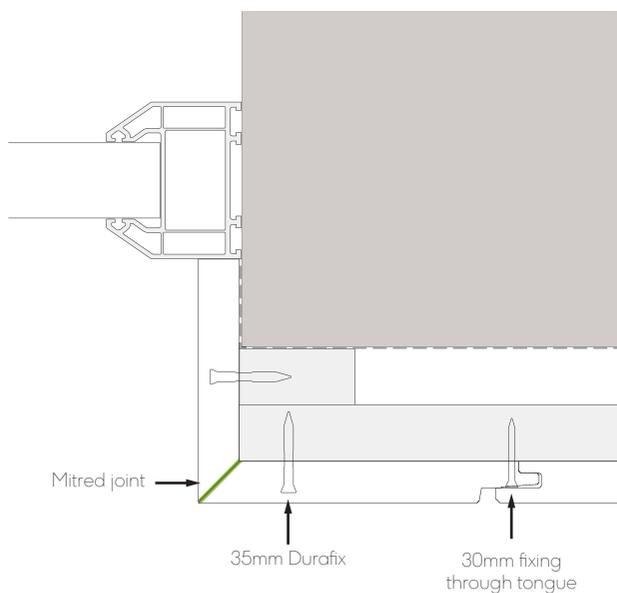
Fig. 13 - Window/door jamb with mitred joint
