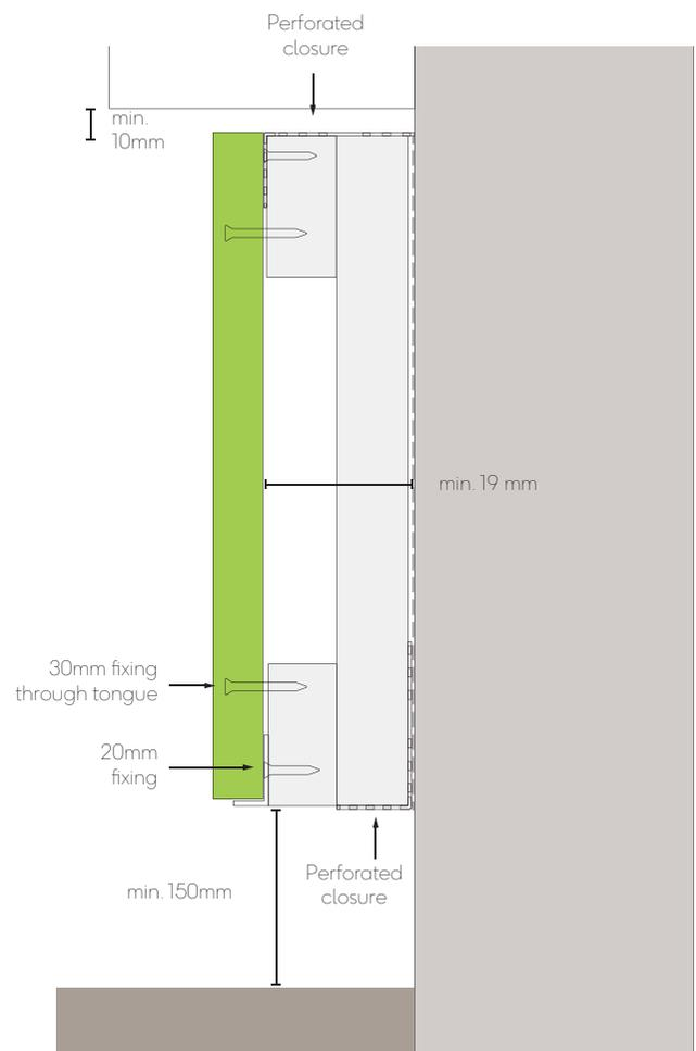
Fig.1 - Top & bottom cladding detail
