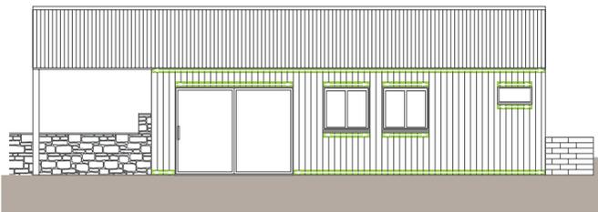
Number of perforated closures = [(width of cladding area x 2) + (width of all windows x 2) + (width of all doors)] / 3
