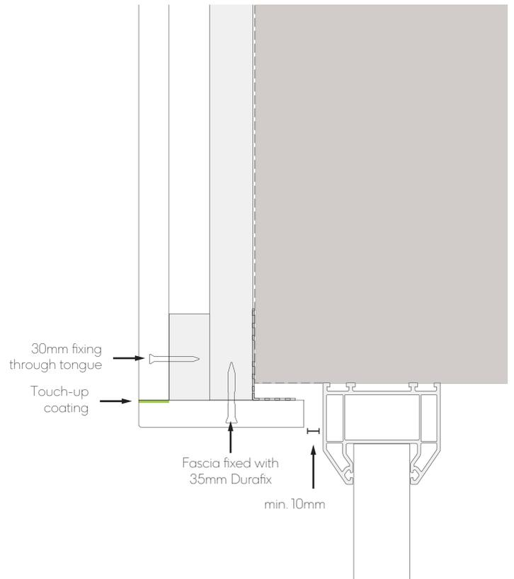
Fig. 12 - Window/door head with fascia
