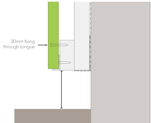
Fig. 17 - First board install
