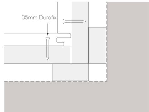
Fig. 9 - Internal butt joint corner detail
