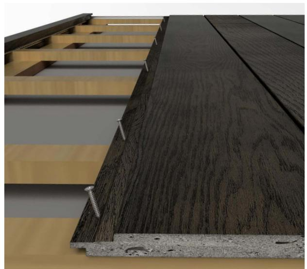
Once the first row of boards have been installed, the second row of boards can be installed beside it, with the groove covering the tongue of the previous board.
