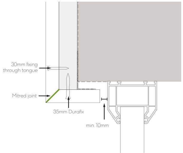
Fig. 14 - Window/door head with mitred joint
